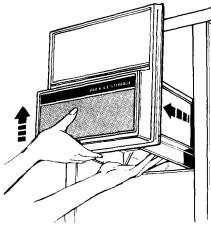
Lift the left corner to free the bin from the shelf, and pull the bin straight out while supporting it at front and back.
